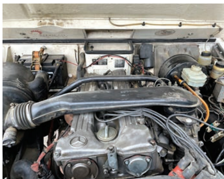
△ M110 straight-six with AMG head makes a strong 220bhp.
