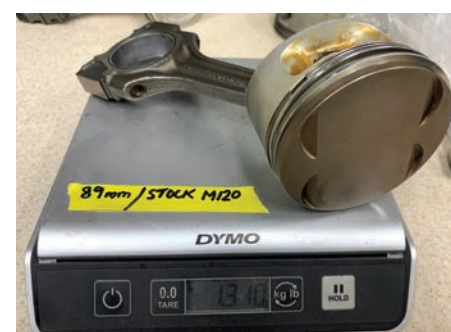
△ A stock, 89mm M120 V12 piston weighs in at 1,310g (1.3kg)...
