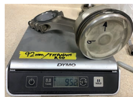
△ ... while RennTech’s titanium 92mm piston and rod is 952g.
