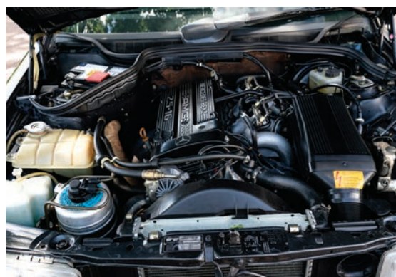
△ Evo's optional AMG Power Pack unlocked 222bhp from the rebored and stroked M102.
